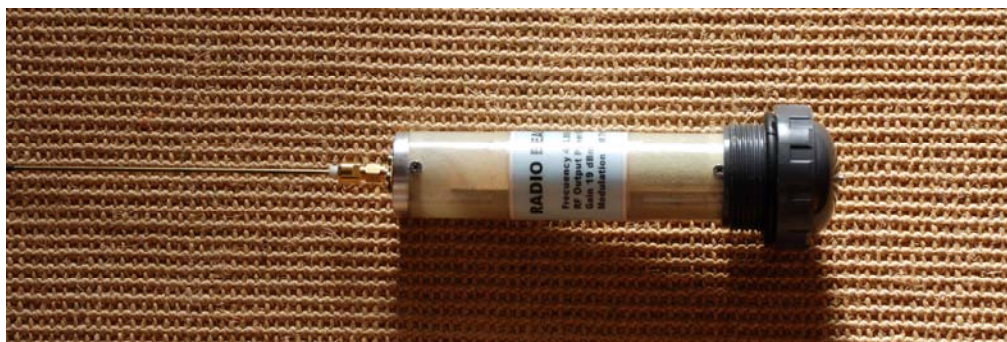
Fig. 35 Emitting module of the nose cone 433 Mhz.
