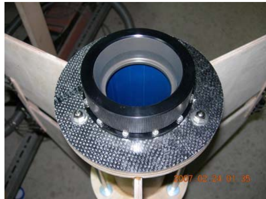
Fig.13 75 mm Aero Pack motor retainer.
