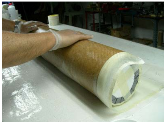
Fig. 18 Second fiber glass laminate.
