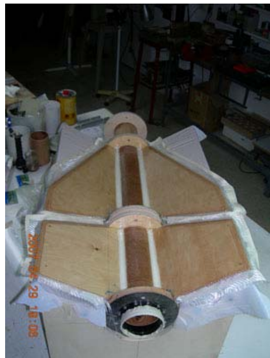
Fig. 10 6 oz. glass cut, and ready to be laminated.
