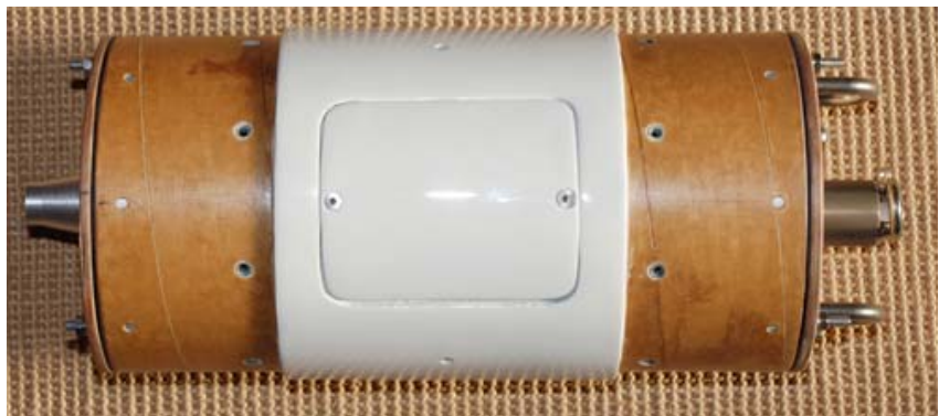
Fig.29 Altimeter bay finished A close up of the M4x20 stainless steel machine screws Din 7991 used to attach the airframe and coupler.
