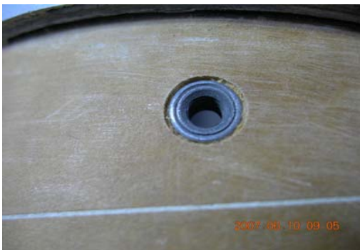
Fig. 25 Riveted nut M4 epoxied.
