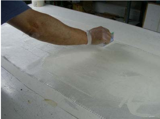
Fig.15 Epoxi impregnating of the 6 Oz fiber glass.
