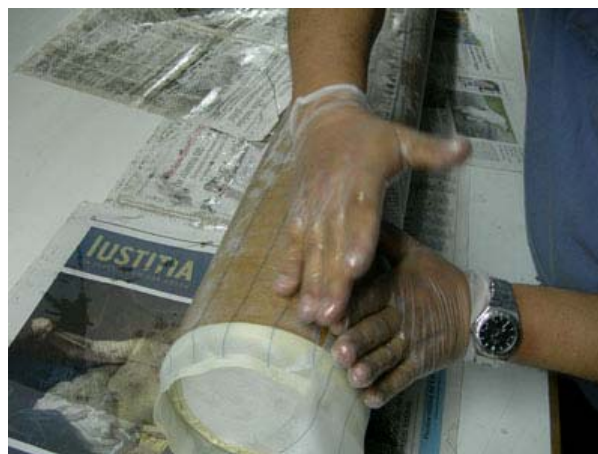
Fig. 19 Rolled of pil ply for better finished final.
