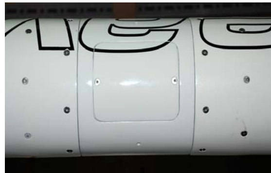
Fig. 26 A close up of the 32 M4 stainless machine screws Din 7991 used to attach the airframe and coupler.
