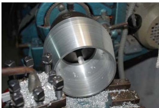
Fig.51 Turned of the tail cone of aluminium.
