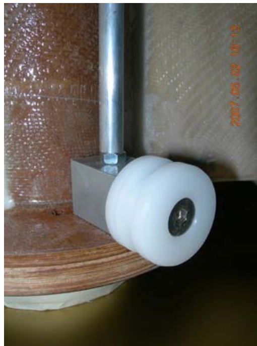
Fig. 14.- Down rail button of Delrin material.
