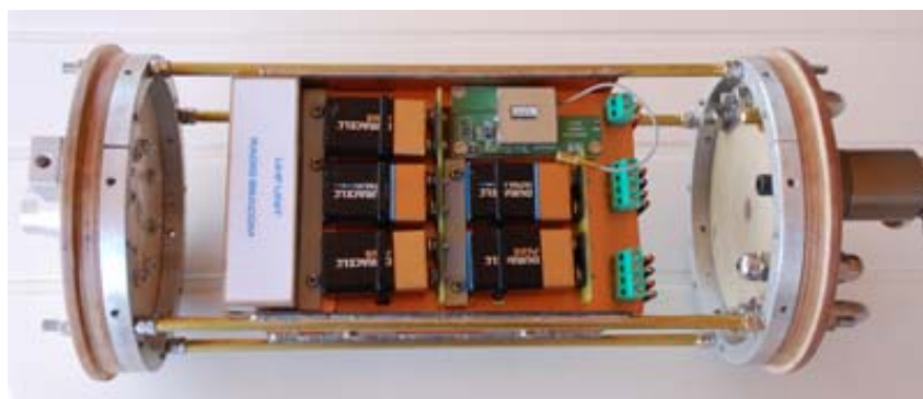
Fig. 27 The internal power section bay, in the left side of the image the rail button support.
