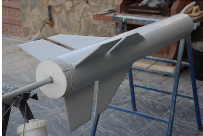
Fig. 53 Painted of the polyurethane primer.
