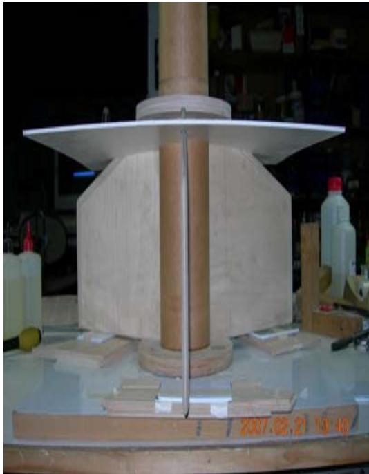
Fig. 7 Aligned down fins and glued of fins and center ring with epoxy.
