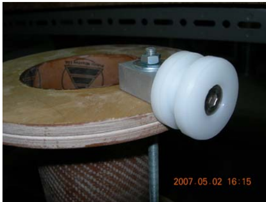
Fig. 12 Upper rail button of Delrin material.
