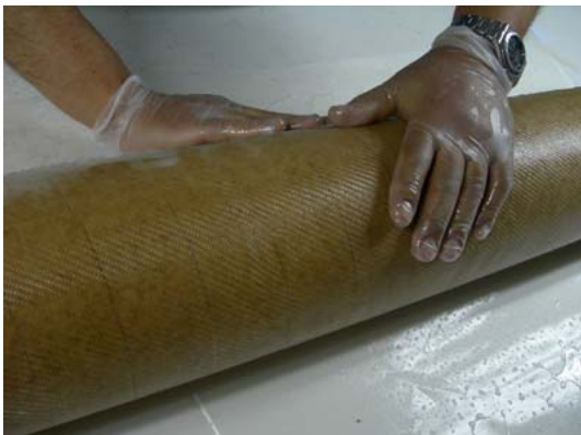
Fig. 17 Adjustment of the fiber glass.
