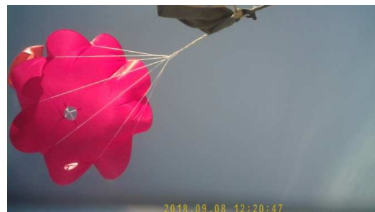
Deployment of the Drogue parachute (Frames on the lower board)
