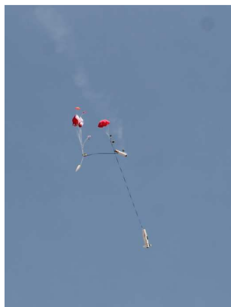
Descent with the Drogue and subsequent start of ejection of the Main's (photos by Alejandro Amor)
