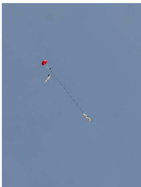
Descent with the Drogue and subsequent start of ejection of the Main's (photos by Alejandro Amor)
