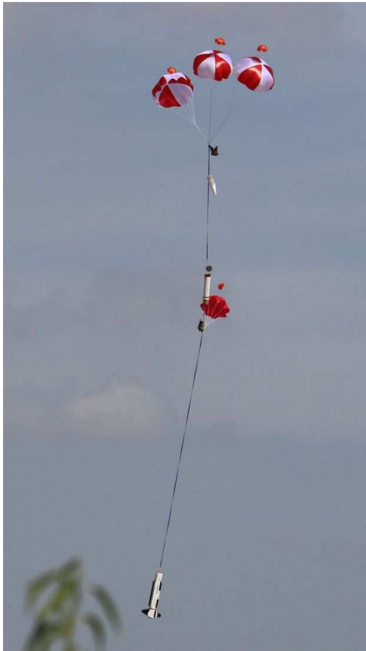
Landing: All the parachutes deployed with their respective pilot parachutes.
